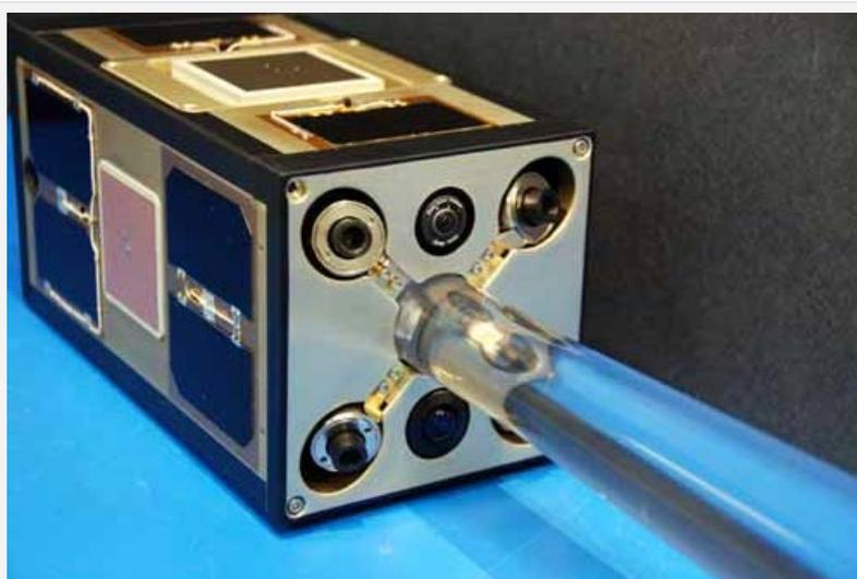
Model of the Aerospace PicoSat Solar Cell Testbed Satellite-2, which will be displayed with the space shuttle Atlantis. (Aerospace image.)
