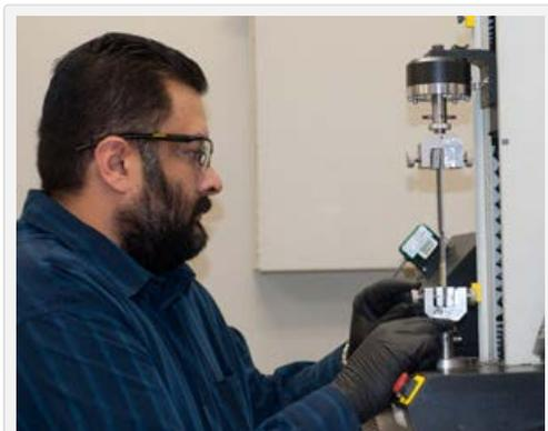
Dhruv Patel performs a lap shear test to determine the mechanical strength of bonded joints that have been prepared using atmospheric plasma treatment. Photo by Eric Hamburg
