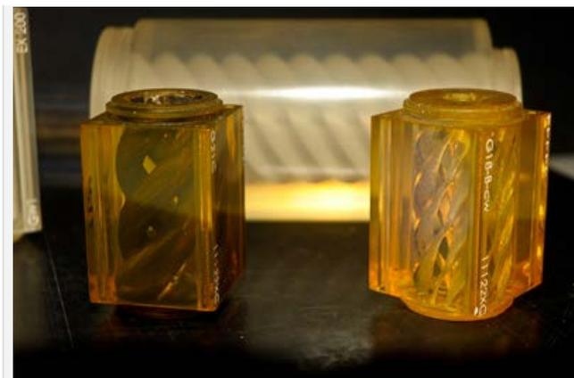
A selection of burned and unburned fuel grains manufactured with rapid prototyping technology. Photo by Elisa Haber
